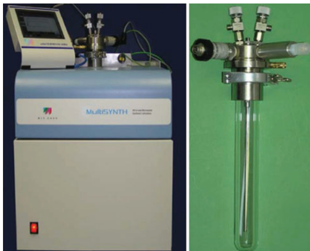
Figure 2 Microwave apparatus multiSYNTH (MLS GmbH, Leutkirch, Germany) with integrated QRS device (left) and the single reactor (right).
