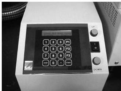
Figure 3. The TraceClean system includes a microprocessor controller for unattended operation.
