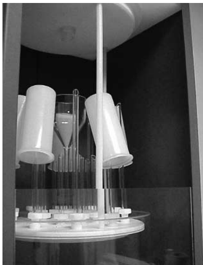
Figure 2. Twenty-position component rack with PTFE-based glass rods.
